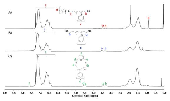
Fig. 3 <sup>1</sup>H-NMR spectra of (A) Pr-PS-4k, (B) *l*-PS-4k, and (C) the corresponding purified *c*-PS-4k (CDCl<sub>3</sub>, 25 °C, 500 MHz).
