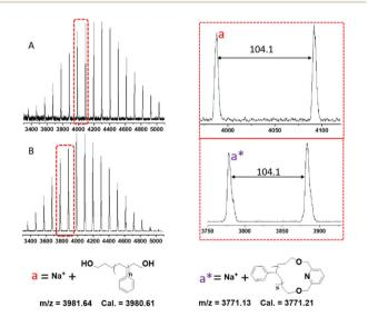
Fig. 6 MALDI-TOF MS of (A) l-PS-4k and (B) c-PS-4k (matrix: dithranol, ionizing agent: NaTFA).
