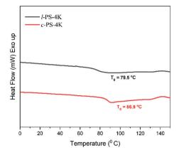
Fig. 8 DSC traces of *l*-PS-4K and purified *c*-PS-4k.
