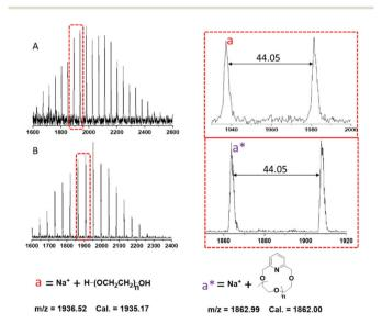
Fig. 7 MALDI TOF MS of (A) I-PEG-2k and (B) c-PEG-2k (matrix: dithranol, ionizing agent: NaTFA).
