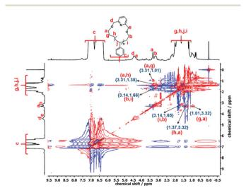
Fig. 5 TOCSY NMR spectrum of c-PS-4k (CDCl<sub>3</sub>, 25 °C, 600 MHz).
