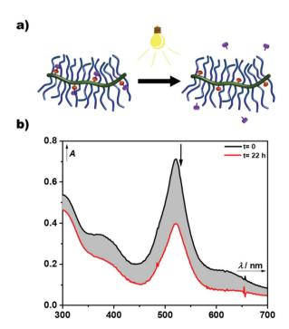
Fig. 7 Photoreaction of the BODIPY decorated poly(organo)phosphazene. (a) Cartoon visualising the light-stimulus controlled release of conjugated phenylacetic acid form the BODIPY decorated polymer carrier. (b) Kinetic study of the photodegradation of the BODIPY decorated poly(organo)phosphazene in MeOH upon 505 nm LED irradiation for the indicated time.
