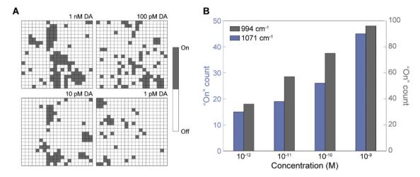
Fig. 6 Digital SERS sensing for the quantitative determination of DA. (A) Digital mapping images with different DA concentrations converted from those in Fig. 5A. (B) Histogram of the total number of "On" spectra using two main peaks for 3-MPBA at 994 and 1071 cm<sup>-1</sup> (the yellow lines in Fig. 5B).
