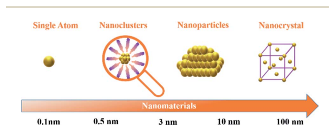
Fig. 1 Size scale from single atoms to nanocrystals.
