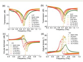
Fig. 4 Experimental results of the THz chiral metasurface sensing filled with different ferromagnetic nanofluids: transmission spectra for (a) the LCP incidence and detection, (b) the RCP incidence and detection, (c) CD spectra, and (d) OA spectra.
