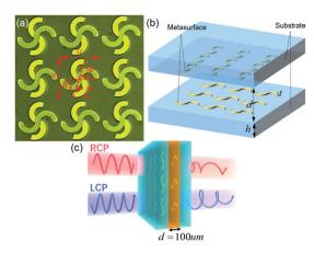
Fig. 2 Geometry of the chiral metasurface: (a) optical micrograph in the top view of the double-layer chiral metasurface; (b) schematic diagram of the metasurface structure, where the nanofluid layer thickness  $d=100~\mu\text{m}$ , the JGS1 glass thickness  $h=500~\mu\text{m}$ , and the metallic structure thickness t=200~nm; (c) schematic diagram of the chiral manipulation for the circularly polarized waves.
