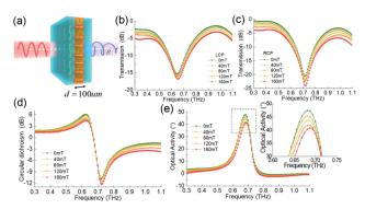
Fig. 7 (a) Schematic diagram of 100 μm thick ferromagnetic nanofluid (16.1%) layer magnetized by the biased magnetic field in the chiral metasurface. Transmission spectra of (b) LCP wave and (c) RCP wave, (d) CD spectra, and (e) OA spectra under the different biased external magnetic fields.
