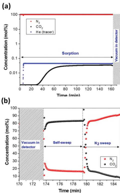
Fig. 25 (a) Breakthrough profile of PEI-functionalised cellulose acetate/silica fibres during  $\text{CO}_2$  adsorption under dry 380 ppm  $\text{CO}_2$ /395 ppm He/balance  $\text{N}_2$  at 35 °C. (b) Concentration profiles during the 'self-sweep' and  $\text{N}_2$  sweep stages of desorption. Reprinted with permission from ref. 39. Copyright (2019) American Chemical Society.
