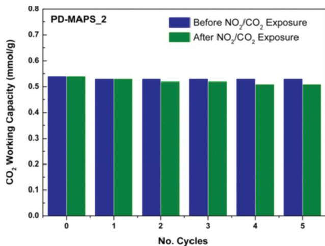
Fig. 23 CO<sub>2</sub> working capacity of the secondary amine-grafted adsorbent before and after exposure to 20 ppm of NO<sub>2</sub> in 10% CO<sub>2</sub>/N<sub>2</sub> at 35 °C. Reprinted with permission from ref. 151. Copyright (2014) American Chemical Society.
