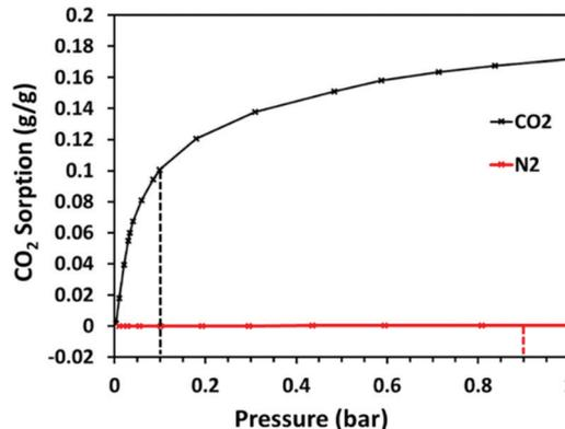
Fig. 16 Selectivity of CO<sub>2</sub> uptake of BC40. Single-component CO<sub>2</sub> and N<sub>2</sub> sorption (g g<sup>-1</sup>) at 90 °C in the low-pressure range. The dashed lines indicate the corresponding interpolated uptakes at the representative pressures of flue gas: 0.10 bar CO<sub>2</sub> and 0.90 bar N<sub>2</sub>. Reprinted with permission from ref. 116. Copyright (2019) American Chemical Society.
