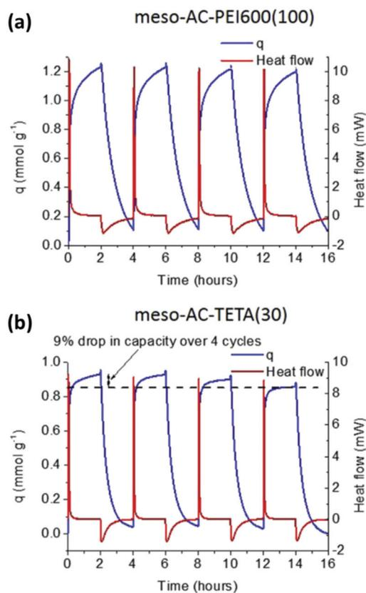
Fig. 18 Cyclic CO<sub>2</sub> adsorption–desorption experiments at 75 °C on (a) meso-AC-PEI600(100), and (b) meso-AC-TETA(30). Reprinted from ref. 130, Copyright (2015), with permission from Elsevier.
