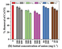
Fig. 7 Effect of co-existing (a) cations, (b) anions on the removal of  $Cr(v_i)$  by **PPY-PANI@RHA**. (Initial  $Cr(v_i)$  concentration: 50 mg  $L^{-1}$ ; contact time: 300 min; agitation speed: 200 rpm; pH ~ 2; temperature: 303 K)
