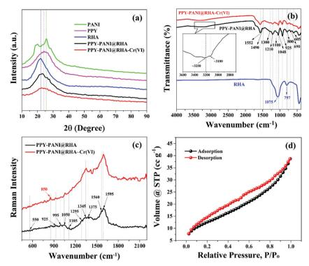
Fig. 3 (a) XRD pattern of PPY-PANI@RHA, PANI, PPY, RHA and PPY-PANI@RHA-Cr(vi) adsorbed composites, (b) FTIR spectra of RHA and PPY-PANI@RHA composites before and after Cr(vi) adsorption, (c) Raman spectra of the PPY-PANI@RHA composite before and after adsorption of Cr(vi), (d) N<sub>2</sub> adsorption-desorption isotherm measured for PPY-PANI@RHA
