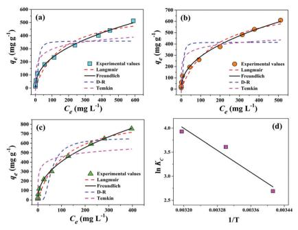
Fig. 6 Experimental data fitted in the Langmuir, Freundlich, D-R, Temkin isotherm model for Cr(vi) adsorption on the PPY-PANI@RHA nanocomposite at (a) 293 K, (b) 303 K, and (c) 313 K temperatures. (d) Van't Hoff plot of InK<sub>C</sub> versus 1/T for Cr(vi) adsorption on PPY-PANI@RHA at a constant adsorbent dose of  $0.8 \text{ g L}^{-1}$  and pH 2.
