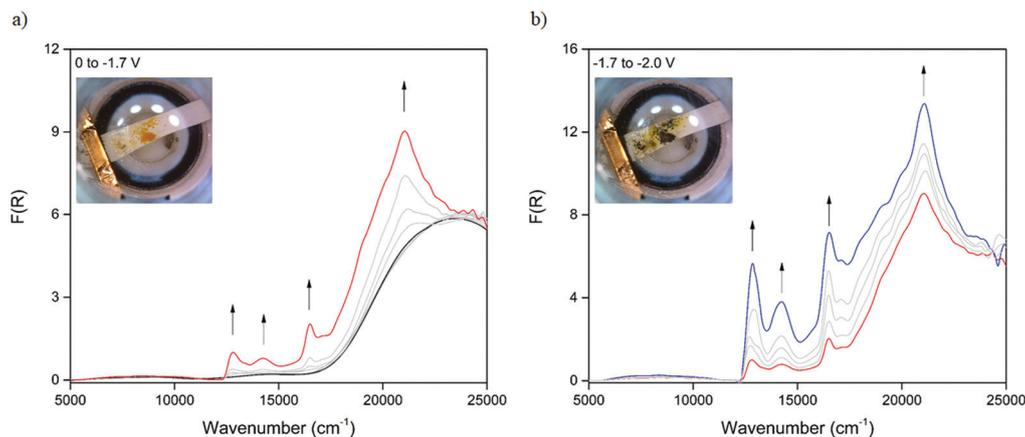
Fig. 2 Solid-state UV-Vis-NIR spectroelectrochemistry of **1** in 0.1 M [(*n*-C<sub>4</sub>H<sub>9</sub>)<sub>4</sub>N]PF<sub>6</sub>/DMF electrolyte showing potential changes from (a) 0 to -1.2 V and (b) -1.2 to -2.0 V where the arrows indicate the direction of the spectral progression. The step at 12 500 cm<sup>-1</sup> is due to a detector change. Insets: Photographs of the sample acquired *in situ* during the time-course of the experiment.
