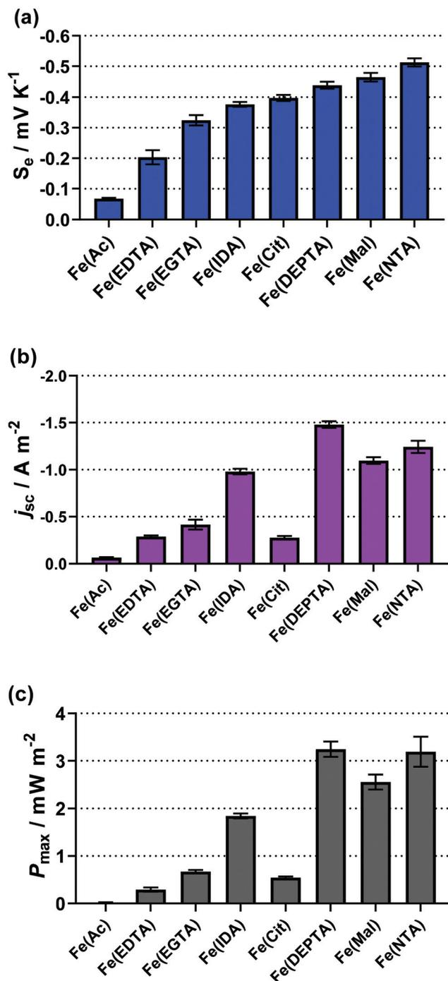
Fig. 3 Bar charts showing (a) the observed Seebeck coefficient ( $S_e$ ), (b) the short-circuit current density ( $j_{sc}$ ) and (c) the maximum power density ( $P_{max}$ ) for the semi-optimised Fe(ligand) systems, visually displaying the values in Table 1.
