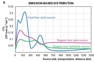
Fig. 6 Emission-based distribution of source-sink transport amount and distance of European CO2. (a) Cumulative emission-based distribution of source-sink CO<sub>2</sub> transportation distances from the 10 prospective CO<sub>2</sub> storage sites reported in Fig. 3. (b) Emission-based distribution of sourcesink CO<sub>2</sub> transportation distances.
