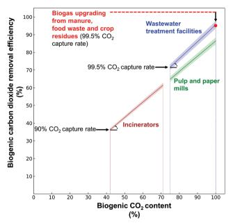
Fig. 1 Biogenic  $CO_2$  content and biogenic carbon dioxide removal efficiencies from different BECCS technology chains. Solid lines represent the average scenario of  $CO_2$  losses in transport and injection; shaded areas show the estimated range of  $CO_2$  losses during transport and injection. Depending on the amount of biomass co-fired, biogenic  $CO_2$  content in biomass co-fired power plants can vary from 1% to 100%.
