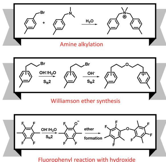
Fig. 14 Several cross-linking pathways of AEMs under high pH conditions.
