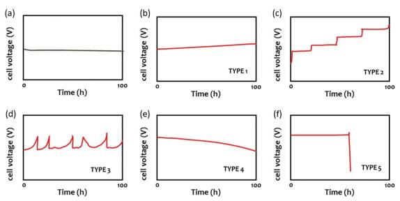
Various voltage behaviors of AEMWEs during 100 hour extended-term test at a constant current density.
