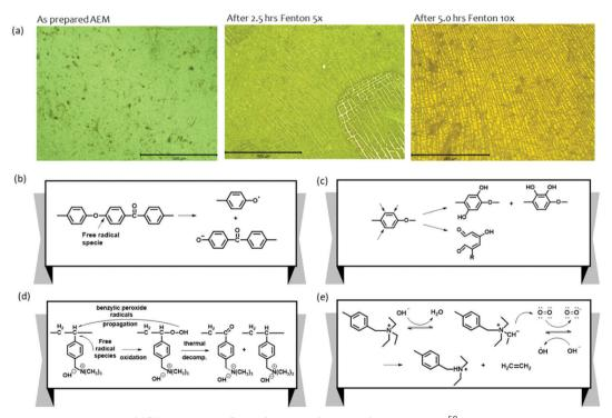
Fig. 13 (a) Optical microscopy analysis of AEM subjected to Fenton's test as a function of exposure time. <sup>58</sup> Major polymer degradation by oxygen radical species. Adapted with permission. <sup>58</sup> Copyright 2013, IOP publishing. (b) Aryl ether polymer backbone degradation. (c) Phenyl group degradation by formation of phenolates. (d) Polymer backbone degradation of quaternized polystyrene (e) Cationic group degradation.
