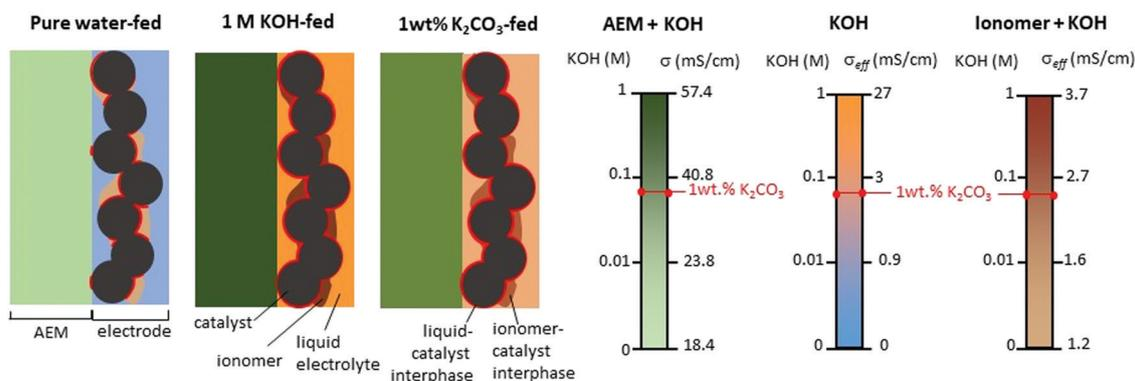
Fig. 3 Schematic illustration of a half cell with supplying pure water, 1 M KOH, or 1 wt%  $K_2CO_3$  solution.<sup>12</sup> We estimated the conductivity of AEM from the high-frequency resistance of the cell using an HTMA-DAPP AEM as a function of KOH concentration at  $50^\circ\text{C}$ .
