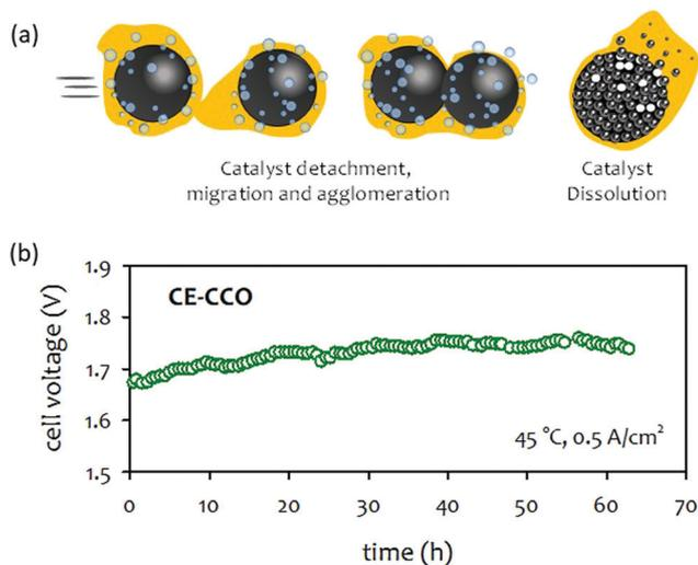
Fig. 15 (a) Catalyst degradation pathways under AEMWE operating conditions. (b) Durability of 1 M KOH-fed AEMWE at  $500 \text{ mA cm}^{-2}$  at  $45 \text{ }^\circ\text{C}$ . AEM: Sustainion<sup>®</sup> X37-50, anode: CuCo-oxide on nickel form (CE-CCO), cathode: Pt/C ( $1 \text{ mg}_{\text{Pt}} \text{ cm}^{-2}$ ).<sup>92</sup> Adapted with permission.<sup>92</sup> Copyright 2020, Elsevier.
