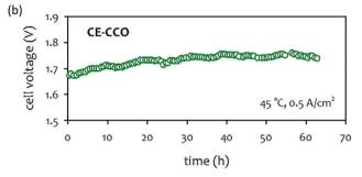
**Fig. 15** (a) Catalyst degradation pathways under AEMWE operating conditions. (b) Durability of 1 M KOH-fed AEMWE at 500 mA cm $^{-2}$  at 45 °C. AEM: Sustainion  $^{(8)}$  X37-50, anode: CuCo-oxide on nickel form (CE-CCO), cathode: Pt/C (1 mg<sub>Pt</sub> cm $^{-2}$ ). Adapted with permission.  $^{92}$  Copyright 2020, Elsevier.
