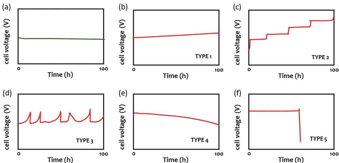
Fig. 6 Various voltage behaviors of AEMWEs during 100 hour extended-term test at a constant current density.
