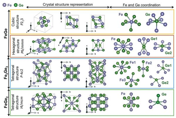
Fig. 3 Crystal structure representations of cubic FeGe, hexagonal FeGe, tetragonal Fe<sub>2</sub>Ge<sub>3</sub> and tetragonal FeGe<sub>2</sub>. Visualized with Vesta<sup>39</sup> with the crystallographic files from ref. 15 and 41-43.
