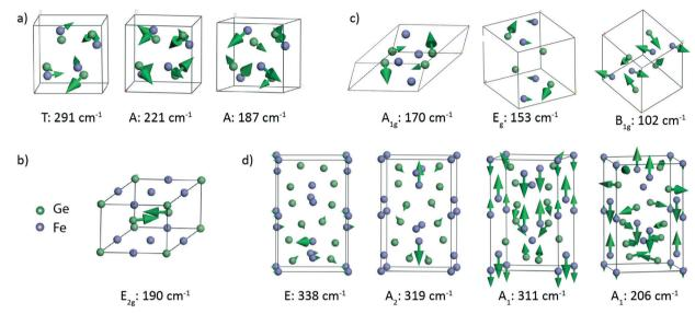
Fig. 4 Representative atomic displacements of the calculated vibrational modes corresponding to a) cubic FeGe phonons at 291, 221 and 187 cm<sup>-1</sup>, b) hexagonal FeGe phonon at 190 cm<sup>-1</sup>, c) FeGe<sub>2</sub> phonons at 170, 153 and 102 cm<sup>-1</sup> and d) Fe<sub>2</sub>Ge<sub>3</sub> phonons at 338, 319, 311 and 206 cm<sup>-1</sup>. The arrows indicate the direction of displacement, and their sizes show the relative amplitudes of the atomic motions.
