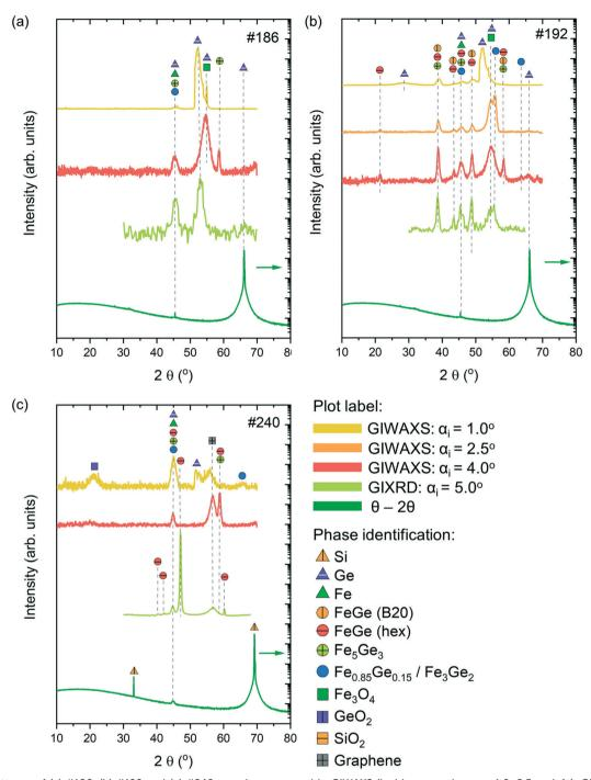
Fig. 6 XRD patterns of (a) #186, (b) #192 and (c) #240 samples measured in GIWAXS (incidence angles  $\alpha_i = 1.0$ , 2.5 and 4°), GIXRD (incidence angle  $\alpha_i = 5.0^\circ$ ) and Bragg-Brentano ( $\theta$ -2 $\theta$ ) configurations, along with the identification of peaks corresponding to different phases. Note that the patterns corresponding to the Bragg-Brentano configuration are presented on the logarithmic scale (pointed with the arrow).
