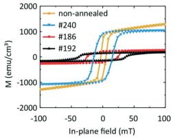
Fig. 9 Comparison of the hysteresis loops for samples #240, #186 and #192 with a non-annealed sample at  $T=100\,$  K. The non-annealed sample contain a nanocrystalline Fe (11.8 nm) layer and an amorphous Ge (19.4 nm) layer.
