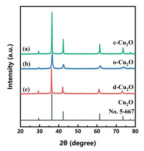
Fig. 6 XRD patterns of (a) c-Cu<sub>2</sub>O, (b) o-Cu<sub>2</sub>O and (c) d-Cu<sub>2</sub>O (synthesized at 40  $^{\circ}$ C). The XRD pattern of standard card of Cu<sub>2</sub>O (JCPDS 5-667) is also shown.
