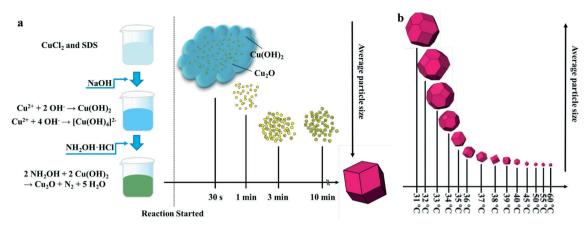
Fig. 1 (a) Schematic diagram of particle size and morphology evolution of  $d-Cu_2O$  with increasing reaction time synthesized at a specific temperature. (b) Schematic diagram of particle size and morphology evolution of  $d-Cu_2O$  with increasing synthesis temperature.
