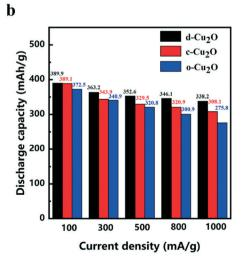
Fig. 7 (a) High rate cycling performance of d-Cu<sub>2</sub>O (reaction temperatures from 31 to 40 °C), c-Cu<sub>2</sub>O and o-Cu<sub>2</sub>O. (b) Discharge capacity of d-Cu<sub>2</sub>O (synthesized at 37 °C), c-Cu<sub>2</sub>O and o-Cu<sub>2</sub>O with the current density ranging from 100 to 1000 mA g<sup>-1</sup>.
