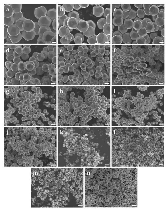
Fig. 5 SEM images of d-Cu<sub>2</sub>O synthesized at different temperatures: (a) 31 °C, (b) 32 °C, (c) 33 °C, (d) 34 °C, (e) 35 °C, (f) 36 °C, (g) 37 °C, (h) 38 °C, (j) 40 °C, (k) 45 °C, (l) 50 °C, (m) 55 °C and (n) 60 °C. Scale bars = 500 nm.
