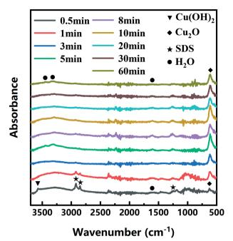
Fig. 3 FTIR spectra of d-Cu<sub>2</sub>O obtained at different reaction times using a 40 °C water bath.
