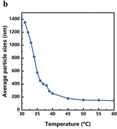
Fig. 4 (a) Reaction time dependence of average particle size of d-Cu<sub>2</sub>O obtained at a synthesis temperature of 40 °C. (b) Reaction temperature dependence of the average particle size of d-Cu<sub>2</sub>O after reaction of 1 h.
