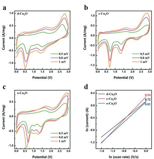
Fig. 8 CV curves of (a) d-Cu<sub>2</sub>O, (b) c-Cu<sub>2</sub>O, and (c) o-Cu<sub>2</sub>O measured at different scanning rates from 0.5 to 1 mV s<sup>-1</sup> after activation at 0.2 mV s<sup>-1</sup> for three cycles. (d) Relationships between ln(current) and ln(scan rate) for d-Cu<sub>2</sub>O, c-Cu<sub>2</sub>O and o-Cu<sub>2</sub>O (peaks of potential at 2.5–3 V).
