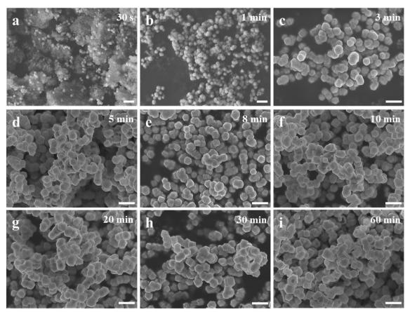
Fig. 2 SEM images of d-Cu<sub>2</sub>O nanoparticles synthesized using a 40 °C water bath with different reaction times: (a) 30 s, (b) 1 min, (c) 3 min, (d) 5 min, (e) 8 min, (f) 10 min, (g) 20 min, (h) 30 min and (i) 60 min. Scale bars = 500 nm.
