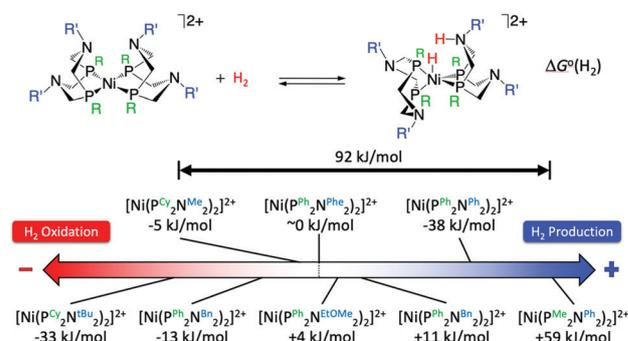
Fig. 6 Standard free energy  $\Delta G^\circ(\text{H}_2)$  for  $\text{H}_2$  addition to various  $[\text{Ni}(\text{P}^{\text{R}}_2\text{N}^{\text{R}'}_2)_2]^{2+}$  complexes. Cy = cyclohexyl, tBu = *tert*-butyl, Me = methyl, Bn = benzyl, Ph = phenyl, Phe = phenyl alanine, EtOMe =  $-\text{CH}_2\text{CH}_2-\text{O}-\text{CH}_3$ . Adapted from Raugé et al.<sup>46</sup>
