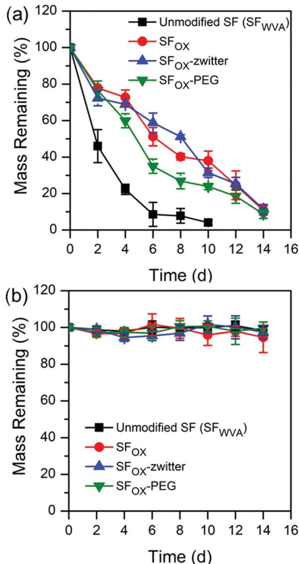
**Fig. 4** Degradation profiles of water annealed silk (**SF<sub>WVA</sub>**), hydroxylated silk (**SF<sub>OX</sub>**), and the silk brush-like polymer films in (a) 1 U mL<sup>-1</sup> protease XIV and (b) 1X PBS, at 37 °C.
