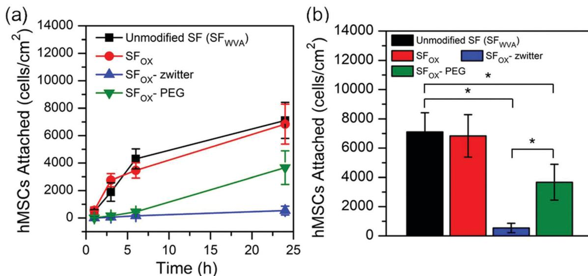
Fig. 6 Attachment (cells per  $\text{cm}^2$ ) of human mesenchymal stem cells (hMSCs) to unmodified silk, oxidized silk, and silk brush-like polymer surfaces normalized to film area at (a) 1 h, 3 h, 6 h, and 24 h; and (b) 24 h. \* denotes significance at  $p < 0.05$ .
