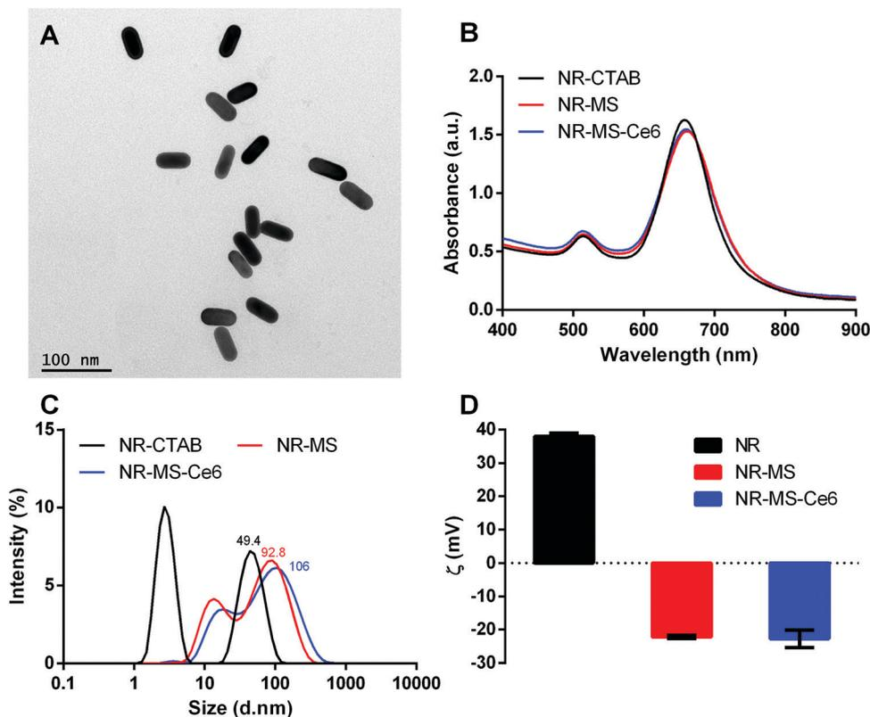
Fig. 2 Characterization of NR-MS-Ce6 and the controls of as-synthesized NR-CTAB and NR-MS showing (A) the monodispersity of the synthesized NR-CTAB used in this study using TEM with 200 000 $\times$  magnification, (B) the UV-vis spectrum, (C) histogram distribution of hydrodynamic diameter ( $D_H$ ) as determined by dynamic light scattering (DLS), and (D) zeta potential of all three samples. Error bars represent standard error for  $N = 3$  samples.
