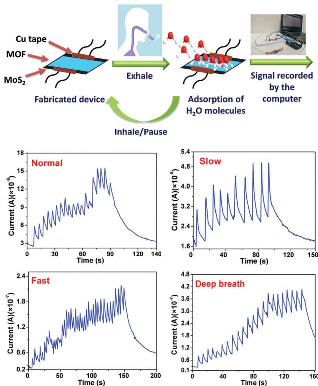
Fig. 3 (top) HKUST-1-MoS<sub>2</sub> fabricated sensor for breath sensing, and (bottom) breath sensing experiments showing variation in the current in response to different types of breaths: normal breath, slow breath, fast breath and deep breath.
