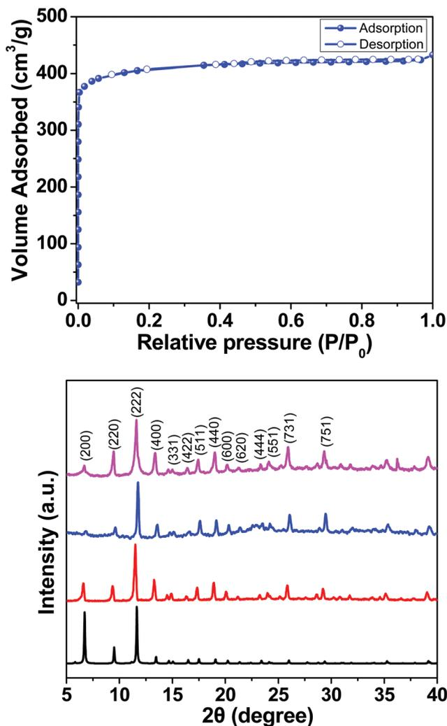
Fig. 1  $N_2$  adsorption isotherm of HKUST-1 (top), and a comparison of the PXRD patterns of the HKUST-1 MOF sample under different conditions (bottom); calculated (black), as-synthesized HKUST-1 crystals (red), the HKUST-1 sample dropcast on  $MoS_2$  (blue), and the HKUST-1 sample after exposure to water for 24 h (pink).
