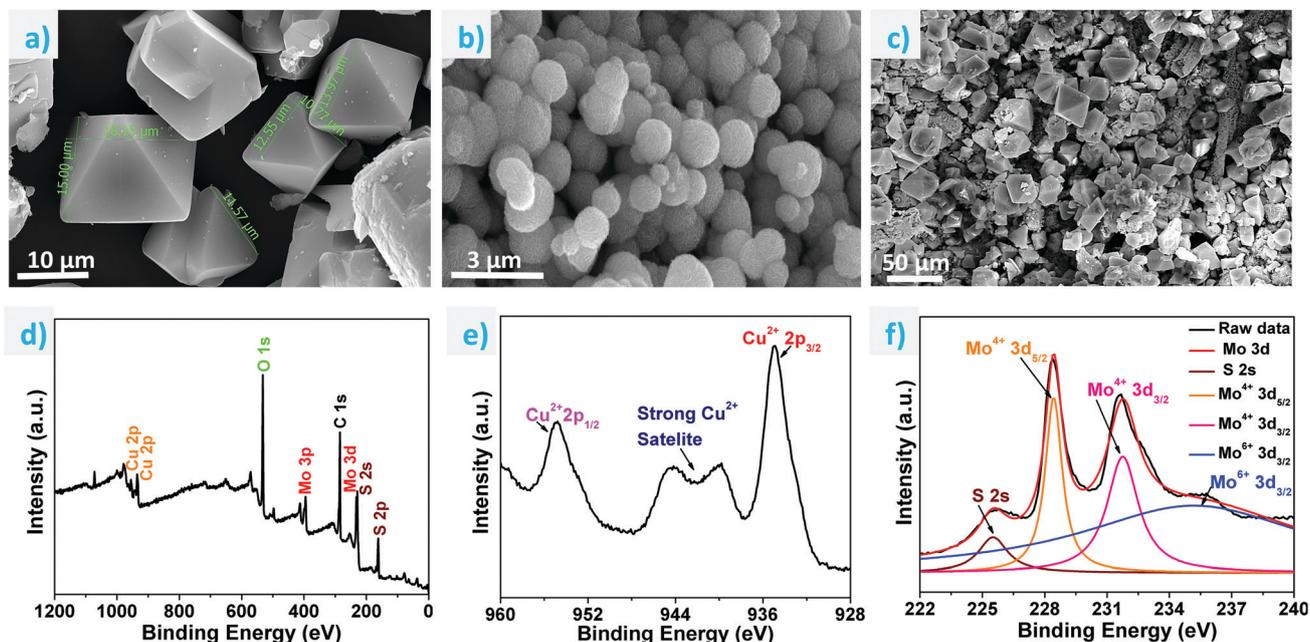
Fig. 2 SEM images of (a) HKUST-1 single crystals, (b) MoS<sub>2</sub>, and (c) HKUST-1 ground sample dropcast on the MoS<sub>2</sub> support, and the XPS data of the HKUST-1–MoS<sub>2</sub> sample; (d) full XPS spectrum; (e) Cu 2p XPS spectrum; and (f) Mo 3d, S 2s XPS spectrum.
