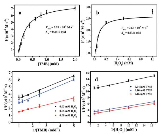
Fig. 5 (a) Steady-state kinetic assay of 2D Fe-BTC at  $0.08 \text{ mM H}_2\text{O}_2$  and different TMB concentrations. (b) Steady-state kinetic assay of 2D Fe-BTC at 0.1 mM TMB and different H<sub>2</sub>O<sub>2</sub> concentrations. (c) Double reciprocal plots of the 2D Fe-BTC activity at 0.08 mM H<sub>2</sub>O<sub>2</sub> and varied TMB concentration. (d) Double reciprocal plots of the 2D Fe-BTC activity at 0.1 mM TMB and varied H<sub>2</sub>O<sub>2</sub> concentration.
