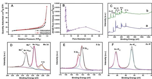
Fig. 5 (A) N<sub>2</sub> adsorption–desorption isotherms and (B) the pore size distribution curve of PPy@MoS<sub>2</sub>, (C) XPS full spectrum of PPy@MoS<sub>2</sub> (a, blue line) and PPy@MoS<sub>2</sub>@Au (b, green line), (D) XPS spectra of Mo 3d of PPy@MoS<sub>2</sub>@Au, (E) XPS spectra of S 2p of PPy@MoS<sub>2</sub>@Au and (F) XPS spectra of Au 4f of PPy@MoS<sub>2</sub>@Au.
