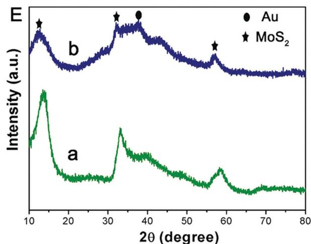
Fig. 2 SEM and TEM images of PPy@ $\text{MoS}_2$  (A and B) and PPy@ $\text{MoS}_2$ @Au (C and D) and (E) XRD patterns of PPy@ $\text{MoS}_2$  (a) and PPy@ $\text{MoS}_2$ @Au (b). Scale bars: 1  $\mu\text{m}$  in (A) and 500 nm in (B–D).
