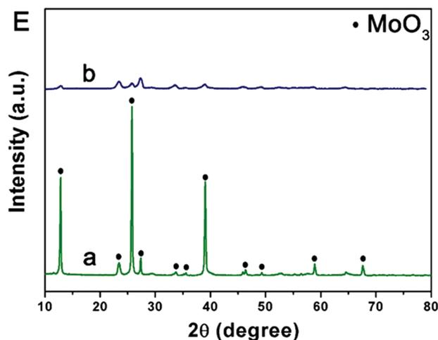
Fig. 1 SEM and TEM images of  $\text{MoO}_3$  (A and B) and  $\text{MoO}_3$ @PPy (C and D), and (E) XRD patterns of  $\text{MoO}_3$  (a) and  $\text{MoO}_3$ @PPy (b). Scale bars: 1  $\mu\text{m}$  in (A–D).
