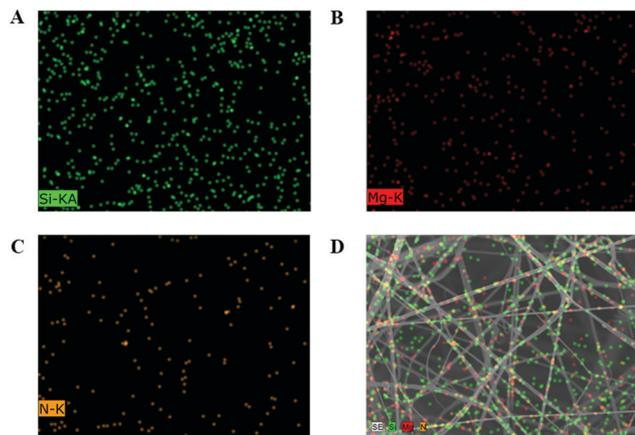
Fig. 3 The energy-dispersive spectroscopy (EDS) images of PLL biofilms: (A) silicon (Si), (B) magnesium (Mg), and (C) nitrogen (N) elements. (D) The merged images of the above three elements with the normal SEM image of the PLL biofilm.
