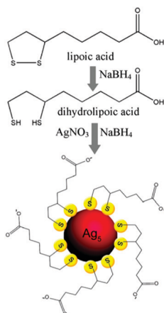
Fig. 7 The formation of an Ag nanocluster–DHLA nanoconjugate. 122
