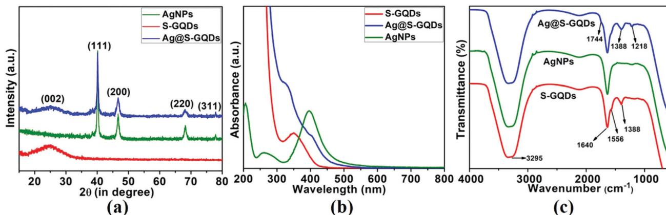
Fig. 2 Illustration of (a) XRD patterns, (b) UV-vis absorption spectra and (c) FTIR spectra of S-GQDs (red lines), AgNPs (green lines) and the Ag@S-GQDs nanocomposite (blue lines).
