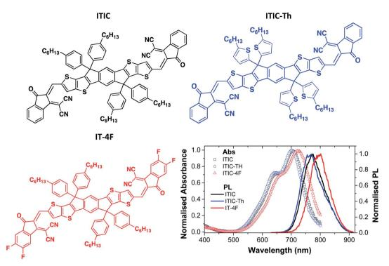
ig. 1 Chemical structures of ITIC derivatives used in this study and their absorption and photoluminescence (PL) spectra.
