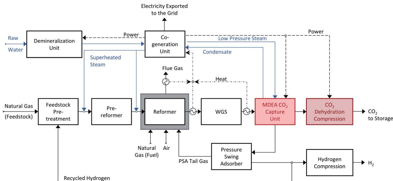
**Scheme 3** Hydrogen production via steam methane reforming with MDEA CO<sub>2</sub> capture. The SMR process scheme is adapted to accommodate the addition of the capture unit before the PSA unit. CO<sub>2</sub> is recovered from the shifted syngas, and subsequently dehydrated and compressed to be suitable for geological storage. The raw hydrogen is purified in the PSA unit and the tail gas is burnt in the external furnace, as in Scheme 1.
