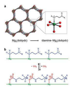
Fig. 1 Structure of diamine-appended variants of the metal-organic framework Mg<sub>2</sub>(dobpdc). (a) Diamines are appended post-synthetically to the open Mg<sup>2+</sup> sites of the framework. (b) Schematic representation of the resulting adsorbents capturing CO2 cooperatively through the formation of ammonium carbamate chains.
