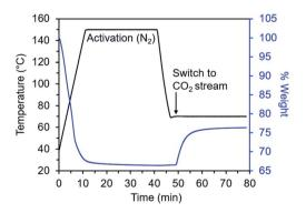
Fig. 2 Overview of TGA adsorption kinetics assay. The diamineappended metal-organic framework sample is activated within a thermogravimetric analyzer under flowing N2 to remove solvent molecules and non-metal-bound diamines from the pores. The sample is then cooled under  $N_2$  to the temperature of interest, the gas flow is switched to a CO<sub>2</sub>-containing stream, and CO<sub>2</sub> adsorption is monitored as a function of time.
