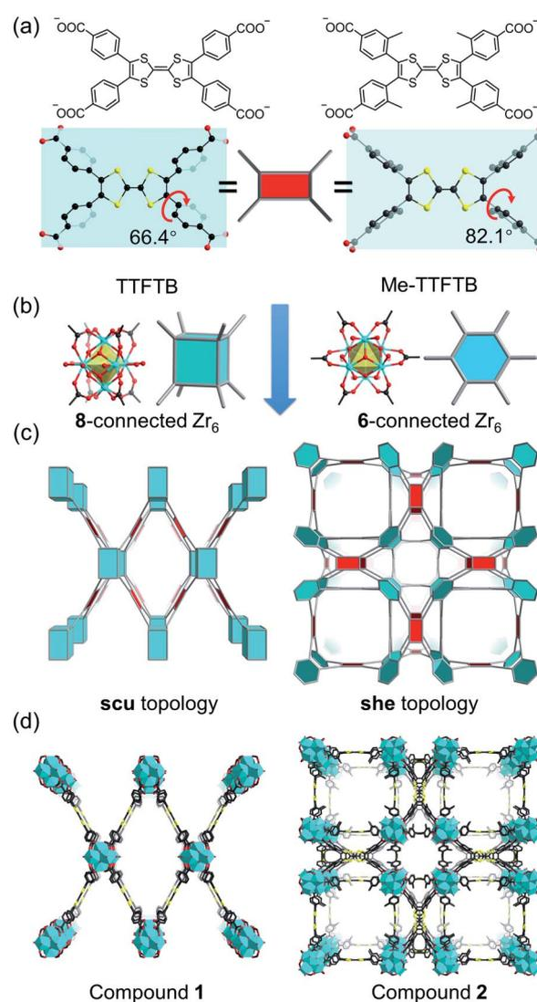
Fig. 1 Topologically guided steric tuning strategy for MOF design (a) TTFTB and Me-TTFTB linkers with different conformations. (b) 8-connected and 6-connected Zr<sub>6</sub> clusters. (c) Targeted topologies formed by Zr<sub>6</sub> clusters and conformationally differing linkers. (d) Crystal structures of compounds 1 and 2. Color scheme: Zr, cyan; O, red; C, black; S, yellow.
