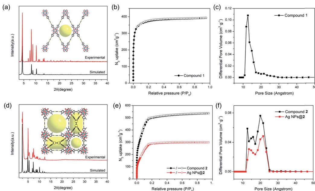
Fig. 2 The experimental and simulated PXRD patterns for compounds **1** (a) and **2** (d) after solvent removal. The  $\text{N}_2$  adsorption–desorption isotherms of compounds **1** (b), **2** and Ag NPs@**2** (e) at 77 K. Pore size distribution of compounds **1** (c), **2** and Ag NPs@**2** (f) calculated from  $\text{N}_2$  adsorption isotherms using a density functional theory (DFT) model.
