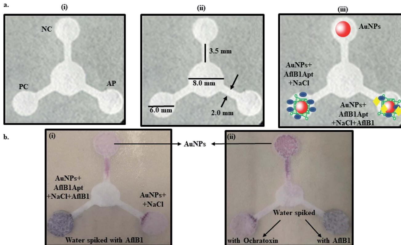
Fig. 4 Schematic representation of  $\mu$ PAD paper microfluidic device. (a) (i) Concept of  $\mu$ PAD—positive control (PC), negative control (NC), analyte pad (AP), (ii) dimensions and (iii) fabrication of the paper device; (b) (i) the color development after spiking Afl B1 in water and (ii) color development in presence of AflB1/no change in color in presence of ochratoxin in water.
