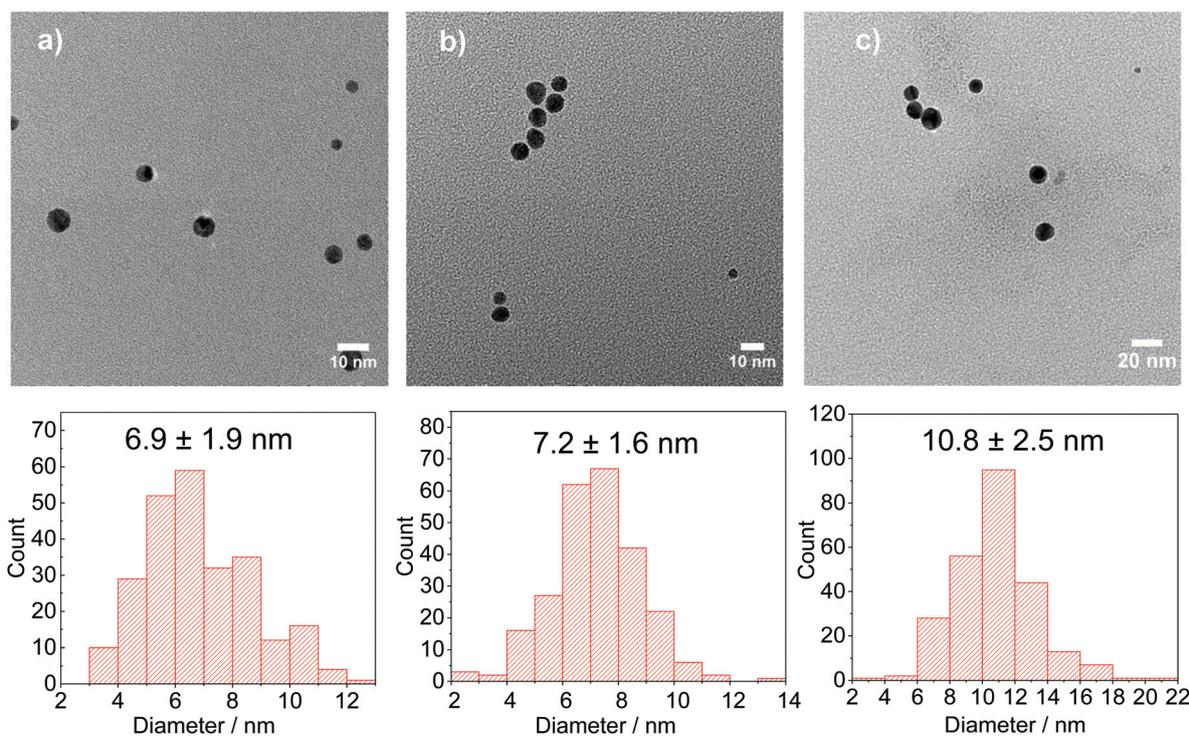
**Fig. 8** Representative TEM images and particle size distribution of Au NPs synthesised using  $\text{AuCl}$  as precursor with a  $\text{DC}^{2-}:\text{Au}$  molar ratio of a. 20 : 1, b. 10 : 1 and c. 1 : 1. Conditions:  $[\text{AuCl}]$ : 0.25 mM,  $[\text{citrate}]$ : 5 mM, pH: 4.4, 80 °C, time: 7 min–11 min.
