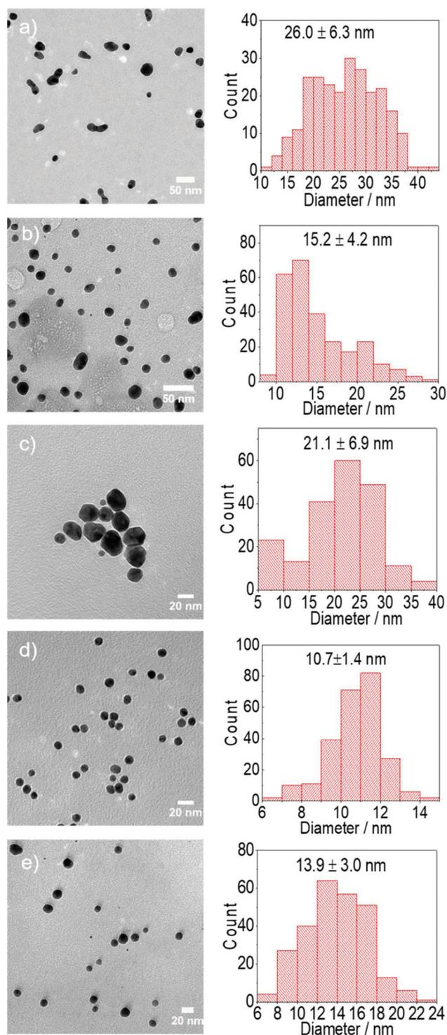
**Fig. 3** Representative TEM images and particle size distribution of Au NPs synthesised using chloroauric acid as the precursor a. [sodium citrate] 2.5 mM at 25 °C, b. [sodium citrate] 2.5 mM at 80 °C, c. [ $\text{DC}^{2-}$ ] 2.5 mM at 25 °C, d. [ $\text{DC}^{2-}$ ] 2.5 mM at 80 °C, e. [sodium citrate] 2.5 mM and [ $\text{DC}^{2-}$ ] 2.5 mM at 80 °C. Conditions: [ $\text{HAuCl}_4$ ]: 0.25 mM, pH: 4.8–4.9, samples are taken after reaction completion.
