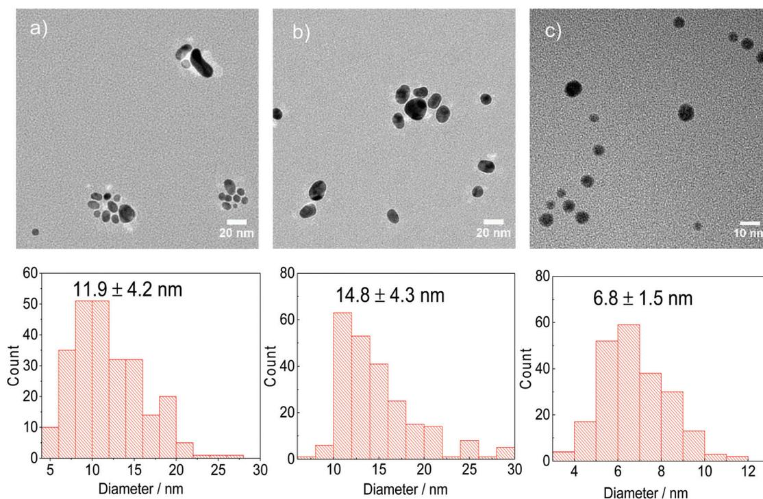
**Fig. 5** Representative TEM images and particle size distribution of Au NPs synthesised using AuCl as the precursor a. in the absence of reducing agent using PVP as stabilizer, b. sodium citrate and c.  $\text{DC}^{2-}$ . Conditions:  $[\text{AuCl}]$ : 0.25 mM, [reducing agent]: 2.5 mM (when applicable), 80 °C pH: 4.8, time: 15–180 min.
