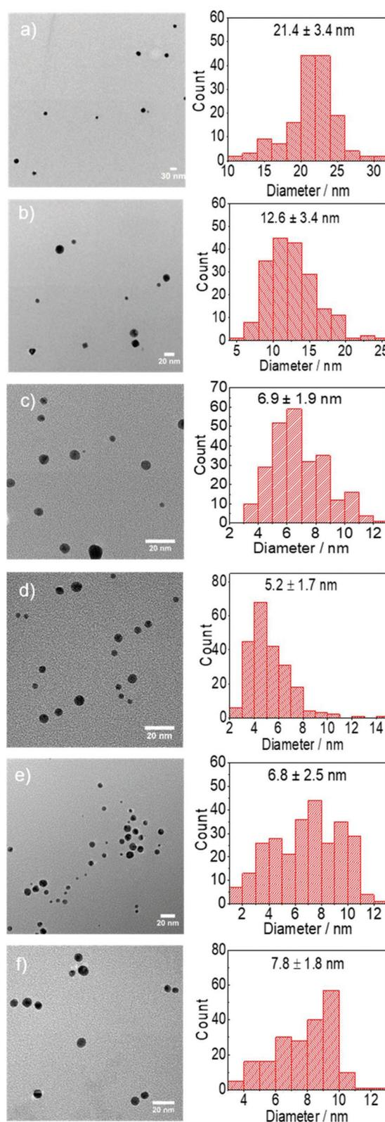
**Fig. 10** Representative TEM images and particle size distribution of Au NPs synthesised using  $\text{AuCl}$  as precursor at pH of a. 2.5, b. 3.6, c. 4.4, d. 6.2, e. 9.0 and f. 9.9. Conditions:  $[\text{AuCl}]$ : 0.25 mM,  $[\text{DC}^{2-}]$ : 5 mM, [citrate]: 5 mM,  $80^\circ\text{C}$ , time: 7 min–13 min.
