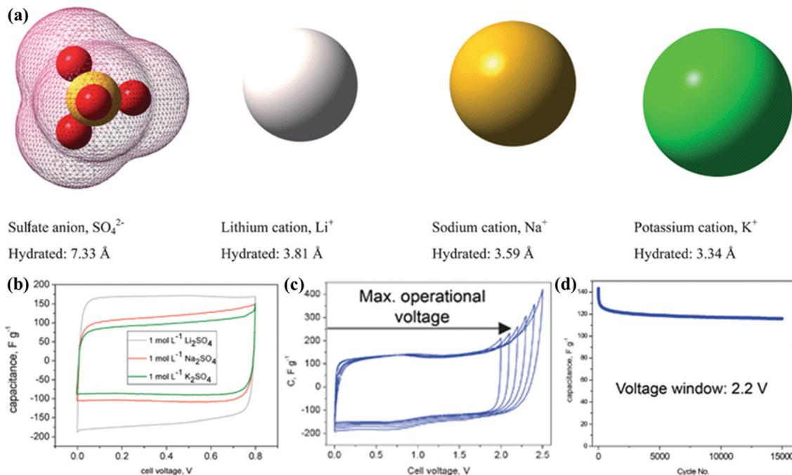
Fig. 11 Ion shapes/dimensions in aqueous solutions (a). Cyclic voltammograms in 1 mol  $\text{L}^{-1}$   $\text{Li}_2\text{SO}_4/\text{Na}_2\text{SO}_4/\text{K}_2\text{SO}_4$  at 1  $\text{mV s}^{-1}$  (b) and 1 mol  $\text{L}^{-1}$   $\text{Li}_2\text{SO}_4$  at 10  $\text{mV s}^{-1}$  (c). Cyclability in 1 mol  $\text{L}^{-1}$   $\text{Li}_2\text{SO}_4$  under 2.2 V (d). (Reproduced with permission.<sup>162</sup> Copyright 2012, The Royal Society of Chemistry.)
