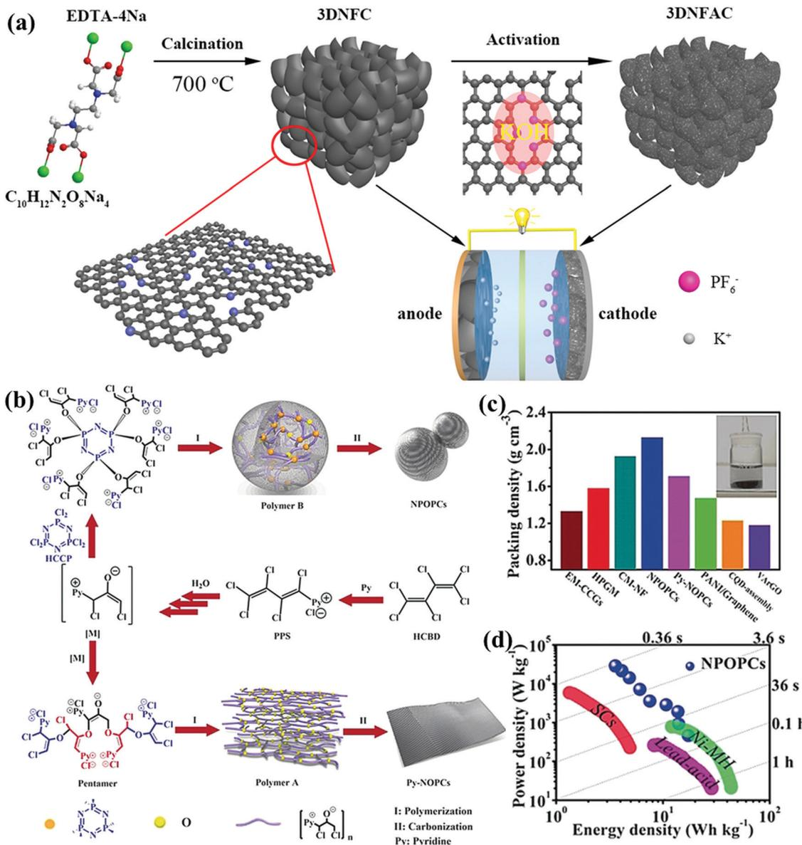
Fig. 9 Schematic illustration of N-rich 3D hierarchical porous carbons (a). (Reproduced with permission.<sup>127</sup> Copyright 2019, Elsevier.) Synthesis of multi-heteroatom-doped porous carbons (b). Packing density (c). Ragone plots (d). (Reproduced with permission.<sup>133</sup> Copyright 2019, Wiley-VCH.)
