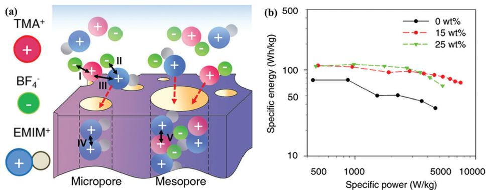
Fig. 13 Schematic of the selective charging behavior of TMABF<sub>4</sub>/EMIMBF<sub>4</sub> ionic mixture electrolyte (a). Ragone plots (b). (Reproduced with permission.<sup>203</sup> Copyright 2017, American Chemical Society.)
