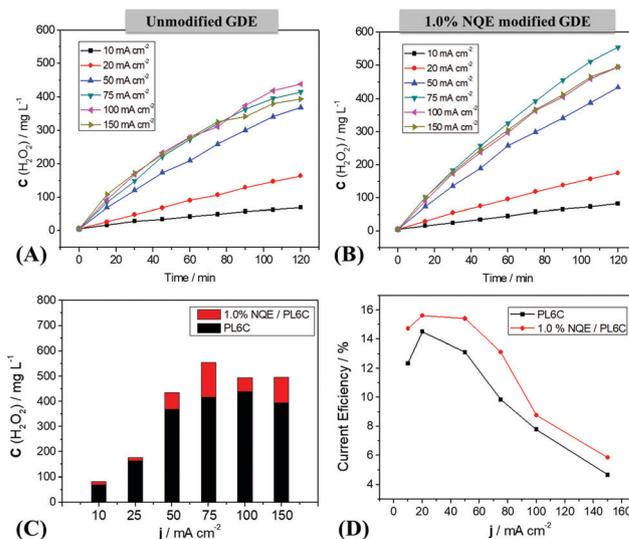
Fig. 3 (A) Electrogenerated  $H_2O_2$  concentration at different current densities on the unmodified GDE and (B) on the 1.0% NQE modified GDE; (C) comparison of the maximum concentration obtained in 120 minutes of electro-synthesis; and (D) current efficiency of all the densities investigated in 0.1 mol L<sup>-1</sup>  $K_2SO_4$  electrolyte, pH = 2.5 ( $H_2SO_4$ ) under 0.2 bar  $O_2$  pressure.
