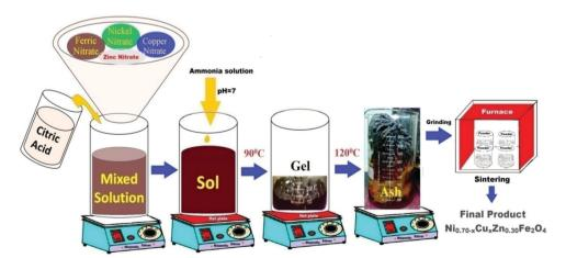
Fig. 1 Schematic of the nitrate-citrate route employed to synthesize  $Ni_{0.70-x}Cu_xZn_{0.30}Fe_2O_4$  (x = 0.00, 0.05, 0.15, and 0.25)
