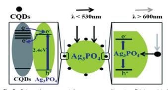
Fig. 5 Schematic representation corresponding to Cdot improved photocatalytic activity of a Cdot/Ag<sub>3</sub>PO<sub>4</sub> complex. Reprinted with permission from ref. 115. Copyright 2012 Royal Society of Chemistry.
