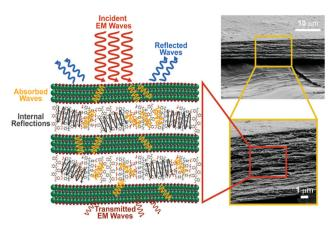
Fig. 6 Schematic of the proposed EMI shielding mechanisms of crosslinked PEDOT:PSS-Ti<sub>3</sub>C<sub>2</sub>T<sub>x</sub> MXene nanocomposite
