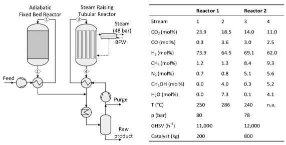
Fig. 9 Simplified scheme and process parameters of the Lurgi two-stage process for methanol synthesis from CO<sub>2</sub> (own illustration based on König and Göhna<sup>194</sup>).
