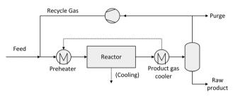
Conventional synthesis loop in methanol, DME and FT-processes.
