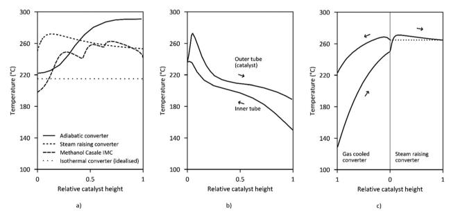
Fig. 7 Temperature profiles along the reactor length of (a) adiabatic converter, steam raising converter, Methanol Casale IMC, and isothermal converter (idealized), (b) Mitsubishi Superconverter, Lurgi MegaMethanol.
