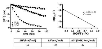
Fig. 2 For the reaction of  $[HPt(depe)_2]^+$  (3) (21.9 mM) with  $CO_2$  (1.0 atm) (top left) concentrations of 3 over time at various temperatures, (top right) corresponding Eyring plot, and (bottom) activation parameters.
