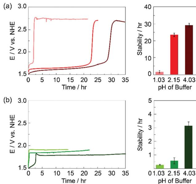
Fig. 3 Stability of  $\text{CoFePbO}_x$  films performing OER at  $1 \text{ mA cm}^{-2}$  in solutions containing (a) 1 M  $\text{KNO}_3$  + 0.1 M  $\text{KP}_i$  and (b) 1 M  $\text{KNO}_3$  + 0.1 M  $\text{KS}_i$  at different pH: 1.03 (light red and light green), pH 2.15 (red and green), and pH 4.03 (dark red and dark green). Representative chronopotentiometry curves (left), and bar graphs indicating average film stabilities (right) at each pH are shown.
