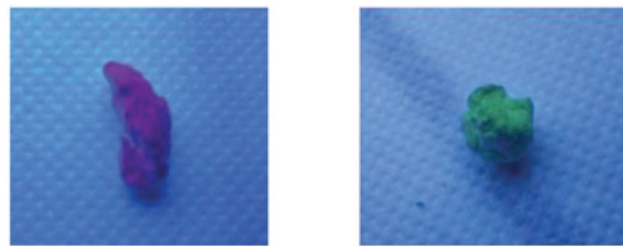
Fig. 8 Polyisoprene rubbers show luminescence under the UV lamp. Reprinted with permission (open access). 50 Copyright 2015 MDPI.
