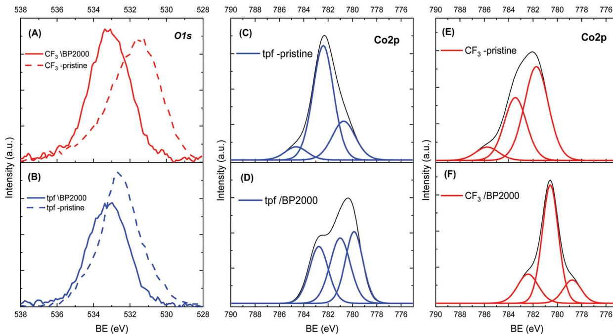
Fig. 3 XPS spectra of (A) O1s of the Co(III)-CF<sub>3</sub>-corrole before and after incorporation in BP2000, (B) O1s of the Co(III)-tpf-corrole before and after incorporation in BP2000, (C) Co2p spectra of Co(III)-tpf-corrole, (D) Co2p of the Co(III)-tpf-corrole after incorporation in BP2000, (E) Co2p spectra of Co(III)-CF<sub>3</sub>-corrole, and (F) Co2p of the Co(III)-CF<sub>3</sub>-corrole after incorporation in BP2000.
