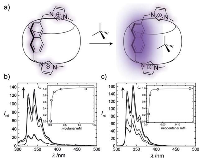
Fig. 3 (a) The encapsulation of a second guest within a Bis·CB8 complex enhances the fluorescence of the first guest; changes in fluorescence can be directly correlated to the binding strength of the second guest. (b) and (c) Changes in fluorescence spectra for Bis2·CB8 complexes, plotted versus wavelength and second guest concentration (inset) for (b) *n*-butane and (c) neopentane.
