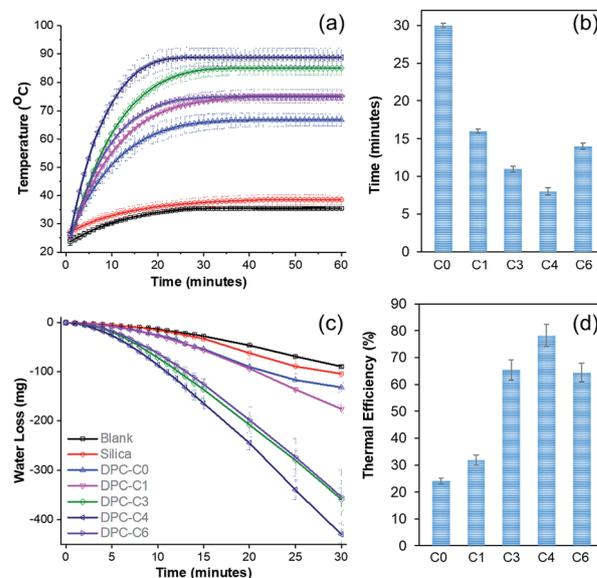
Fig. 4 (a) Temperature of water with time, (b) kinetics of heating (time required to reach  $65^\circ\text{C}$ ), (c) steam generation (loss of water) over time, and (d) thermal efficiency of steam generation by plasmonic DPC-Cx, using visible to NIR light (400 to 1100 nm wavelength).
