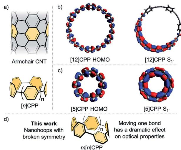
Fig. 1 (a) Structure of an armchair carbon nanotube (CNT) and its relation to [*n*]cycloparaphenylenes; (b) HOMO (left) and excited state (right)  $S_1'$  orbitals of [12]CPP and (c) HOMO (left) and excited state (right)  $S_1'$  orbitals of [5]CPP. Orbitals have been calculated using CAM-B3LYP/STO-3G level of theory. (d) *meta*[*n*]CPPs with broken symmetry in this work.
