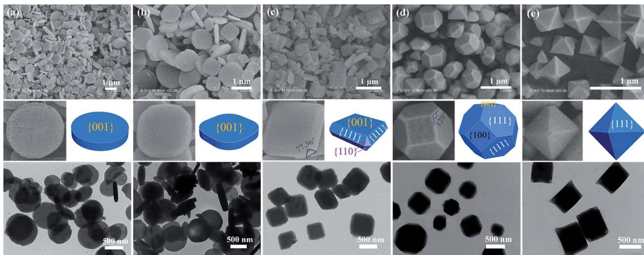
Fig. 2 SEM, enlarged SEM, TEM images and the corresponding 3D geometry models of as-synthesized  $\text{NH}_2\text{-MIL-125(Ti)}$  obtained under different concentrations of CTAB: (a) 0, (b) 1 mM, (c) 2 mM, (d) 3 mM and (e) 4 mM.
