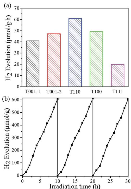
Fig. 4 (a) Photocatalytic hydrogen production using  $\text{NH}_2\text{-MIL-125(Ti)}$  with different morphologies. (b) Recycling tests using T110.
