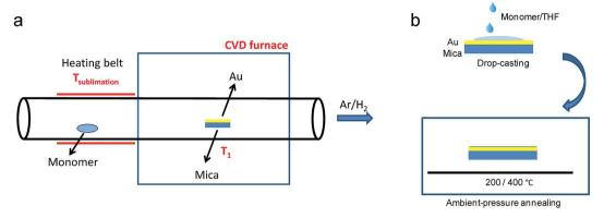
Fig. 4 Schematic illustration comparing GNR synthesis through (a) CVD and (b) solution processing, which avoids the use of heat and vacuum for the monomer deposition. (a) Reproduced with permission. Copyright (2016) American Chemical Society; (b) Reproduced with permission. Copyright (2017) The Chemical Society of Japan.
