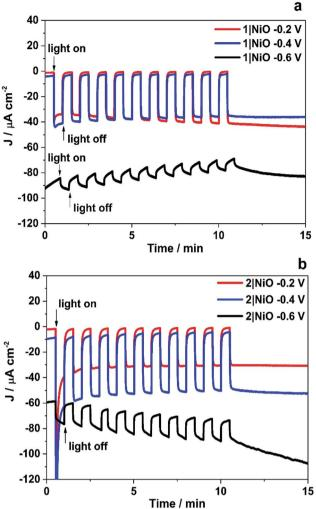
Fig. 7 Chronoamperometry measurements of 1|NiO (a) and 2|NiO (b) immersed in pH 3 buffer containing 0.1 M potassium hydrogen phthalate.  $E_{appl} = -0.2$  V, -0.4 V and -0.6 V vs. Ag/AgCl (3.0 M NaCl). Chopped light illumination was applied with 30 s intervals (10 cycles of dark current/photocurrent).
