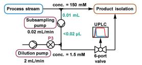
Fig. 5 A schematic representation of the continuous subsampling and dilution setup used for online UPLC analysis, via automated sample injections.
