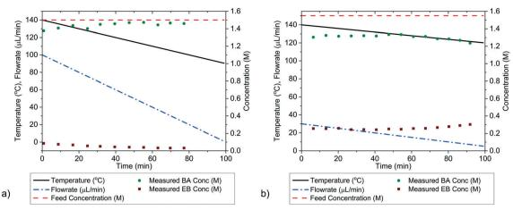
Fig. 8 Control variable profiles and outlet concentrations of benzoic acid (BA) and ethyl benzoate (EB) obtained by automated HPLC measurements for the two-variable transient campaigns, where flowrate and temperature were ramped simultaneously. Figure a) is the "wide spacing" design chosen by the user to cover a wide range of experimental conditions, and figure b) is the "improved" design chosen from screening many designs in simulated experiments.
