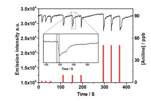
Fig. 3 Time-resolved fluorescence intensity (black line) of a PDI@PVDF fibril film upon consecutive exposures to various concentrations of aniline vapors. (1 s exposures, concentrations indicated by the red columns). Inset: fluorescence change upon exposure to 10 ppb aniline, and the filled rectangle indicated the exposure times (the emission intensity at 630 nm was measured for every 300 ms,  $\lambda_{\rm ex}=365$  nm).
