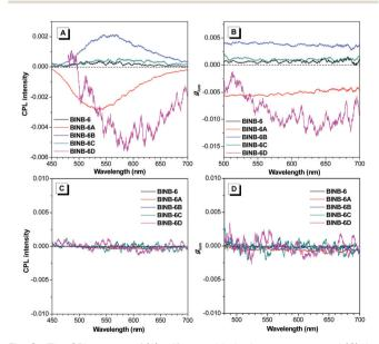
Fig. 6 The CPL spectra of (A) self-assembled microstructures and (C) the solution state of **BINB-6** to **BINB-6D**. The corresponding  $g_{\text{lum}}$  value of (B) self-assembled microstructures and (D) the solution state of **BINB-6** to **BINB-6D**.
