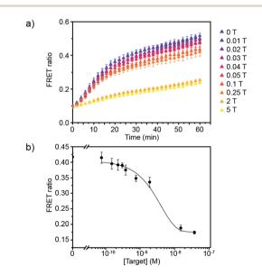
Fig. 3 Evaluation of the sensitivity of the miRNA detection assay. (a) FRET signal traces over time in the presence of various mole equivalent of target miR-29a (1 T corresponds to  $7.6 \times 10^{-9}$  M). (b) Corresponding dose–response curve obtained after 30 min of incubating Dil and DiD liposomes together at 37 °C (liposome concentration of  $1 \times 10^{-4}$  M). (n=3).
