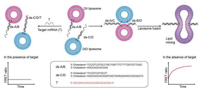
Fig. 1 Schematic illustration of miRNA detection assay based on inhibition of DNA-mediated liposome fusion. Target miRNA (red strand, miR-29a) is complementary to the toehold on ds-C/D and hybridises to it, blocking liposome fusion. In the absence of target, liposome fusion is promoted by ds-A/B and ds-C/D hybridising in a zipper-like manner.
