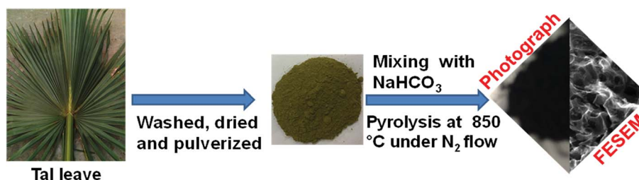
Scheme 1 Schematic representation for the preparation of PTPCNs from tal leaves at 850^\circ\text{C} .
